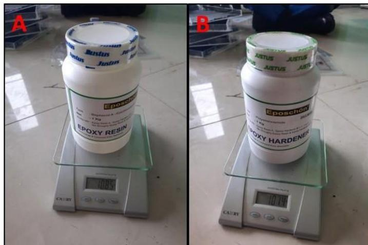
**Gambar 5.** (a) Penimbangan *epoxy resin* (b) Penimbangan *epoxy hardener*
